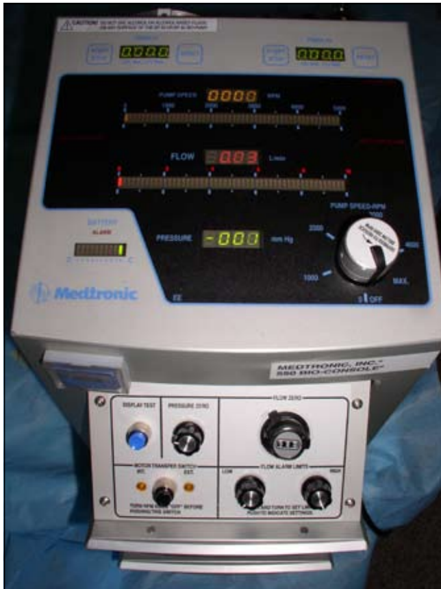
Fig 2. Photograph of the console of the Biomedicus pump (Medtronic Inc), two independent consoles controlled the Biomedicus pumps for flow and revolutions per minute.
