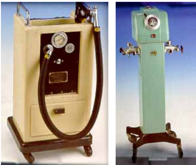
Fig 11. The Minnitt (left) and the Lucy Baldwin (right) apparatus
