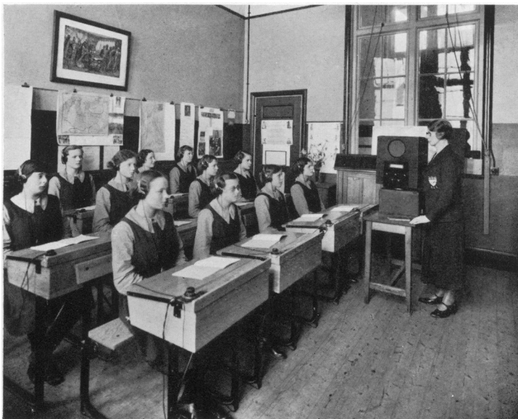
Fig. 5—VALVE AMPLIFIER WITH MULTIPLE EARPHONES IN USE IN A SCHOOL FOR DEAF CHILDREN.
